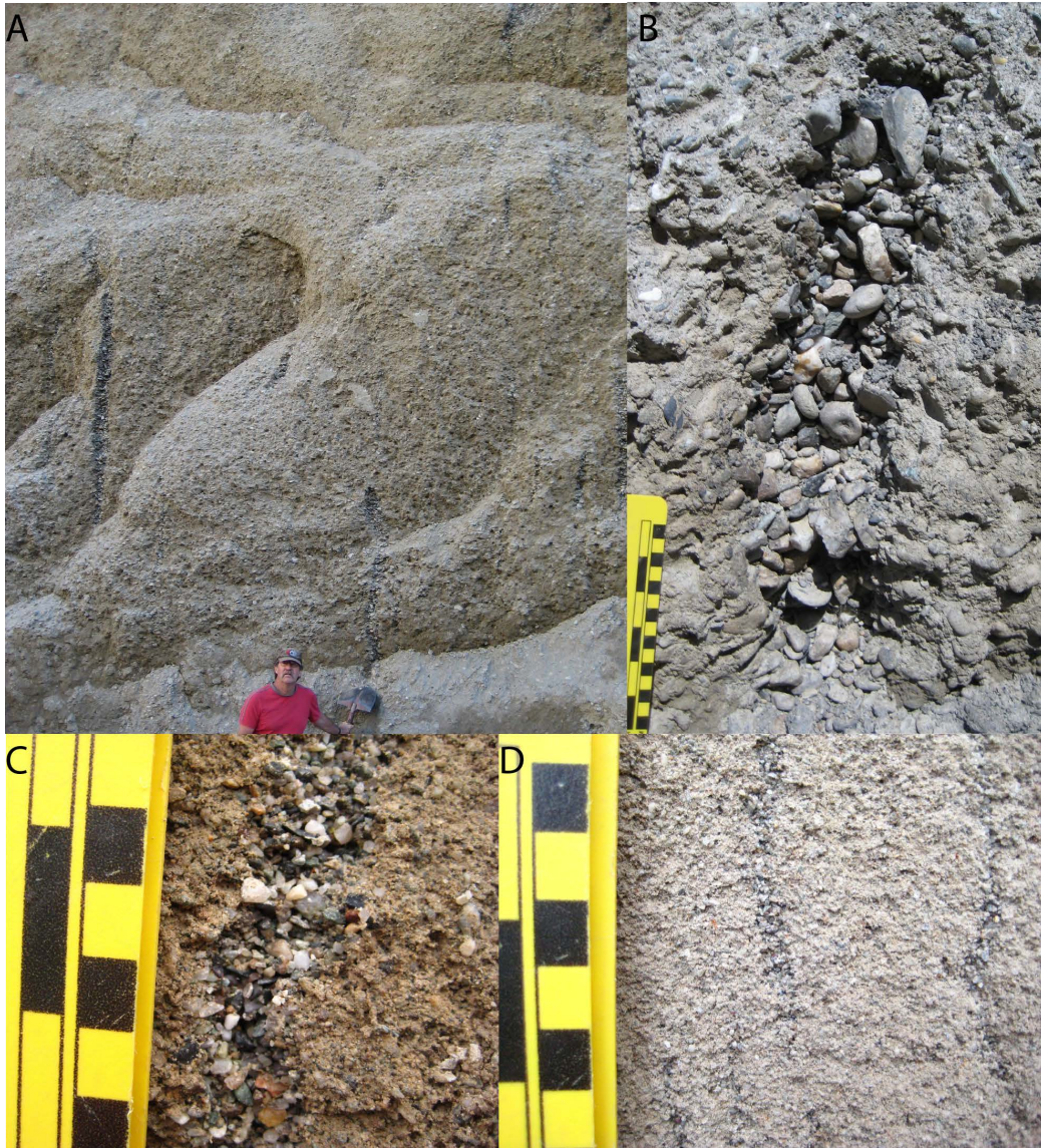
Figure 2.10. Pavoni pipes in Bonaduz gravel at the Reichenau quarry. A) Pipes in the lowest exposed gravels. B) A single pipe showing the absence of silt and sand within the gravel, and steeply dipping stones. C) Pipe with granule-size particles. D) Pipes near the top of the quarry dominated by coarse sand-size particles.
